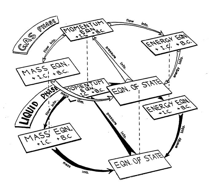
FIGURE 1 : Schematic Of Information Flow In Two-phase Flow Models
