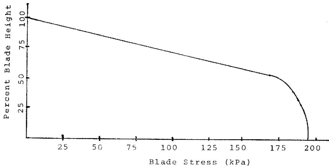
Stress Profile In Long Turbine Blade
