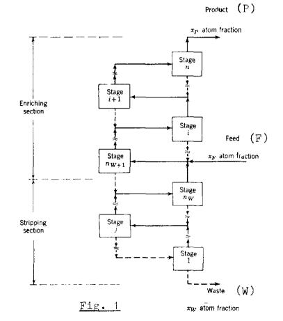
and waste end is called the <u>stripping section</u>, used to increase the recovery of the desired isotope from the feed. Stages of the cascade are numbered consecutively from 1 at the waste end of the plant to n at the product end. The highest stage of the stripping section is numbered  $n_{\rm W} \cdot$
