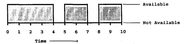
Both reliability and availability are unit-less: reliability is a probability and availability is a fraction. Note, however, that for the system shown in the figure above, if you pick a time in the figure at random, the probability that the system will be working at that time is 0.8.
