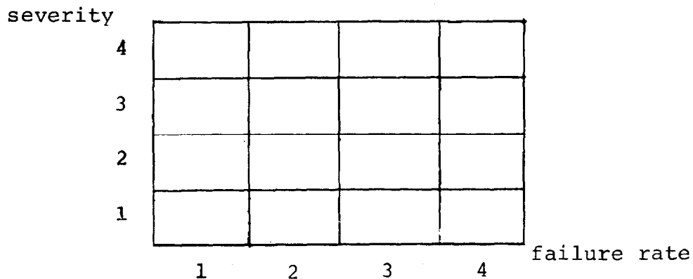
Figure 1: Typical Grid for FMECA
