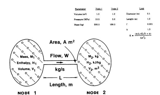
Figure 5.1 Simple 2-node, 1-link system.
