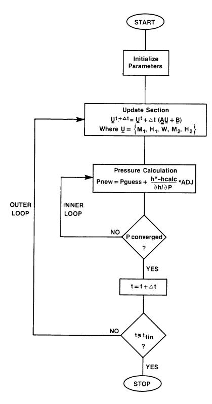
Figure 5.2 Program flow diagram for the normal method.
