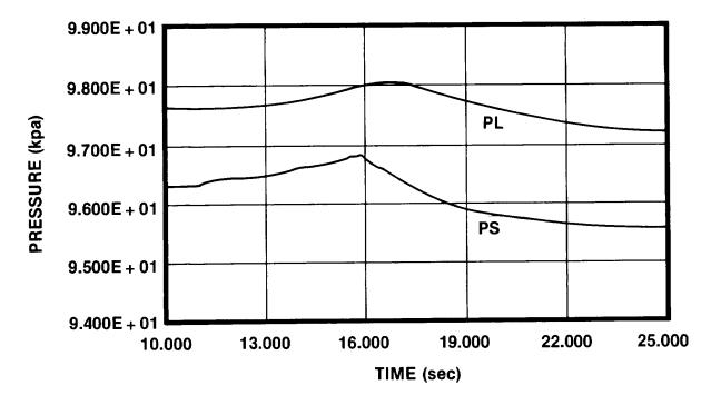
Figure 5.8 Pressurizer's pressure transient for the parmalmethod with error tolerance of 0.2%.
