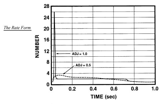
**Figure 5.4** Number of iterations per pressure routine call for the normal method with a time step of 0.01 seconds and a pressure error tolerance of 0.001 of full scale (10 mPa).
