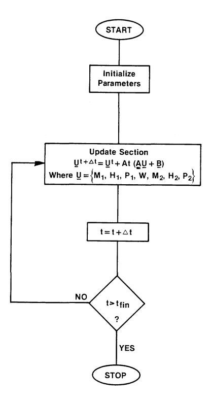
Figure 5.3 Program flow diagram for the rate method.
