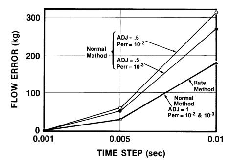
**Figure 5.5** Integrated flow error for the rate method and the normal method for various fixed time steps, convergence tolerances and adjustment factors.
