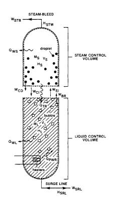
**Figure 5.7** Schematic of control volumes in the pressurizer.
